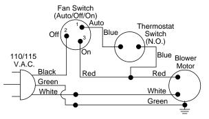
Figure 19 - Wiring Diagram For Fan Accessory Built-In Installation
